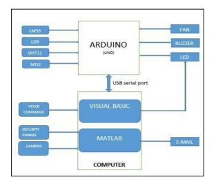
Fig 1.1.A block diagram representing the circuit developed
